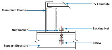
Fig 5: Modules Installed with Screw Fitting Method
