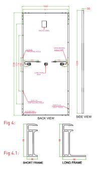
Fig 4: Mechanical Drawing of PV module SOMERA VSMH.78 AAA.05, SOMERA VSMHBB.78.AAA.05 and PREXOS VSMDHT.78.AAA.05
